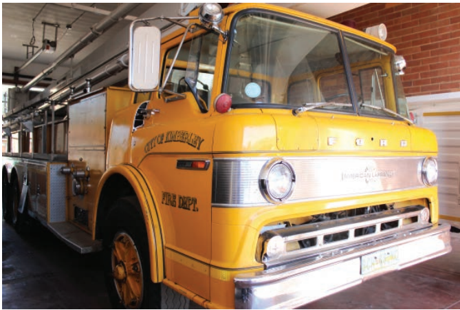
The 1980 model Ford Snorkel hydraulic platform
